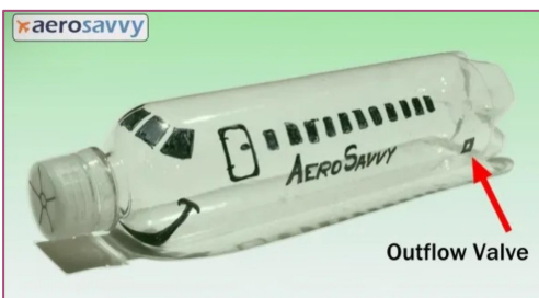
The outflow valve on the fuselage of a plane is similar to a water bottle with a little hole in its side. By varying the size of the hole, we can regulate the pressure inside the cabin of the plane.
