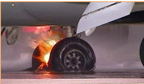
A plane's wheel on fire as a result of friction causing and increase in its temperature.
